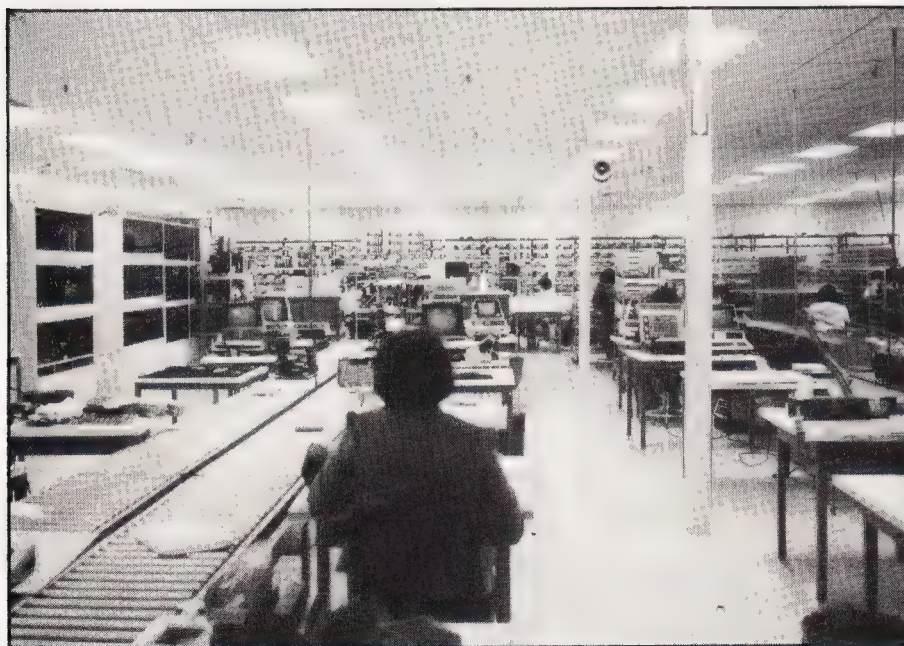
The other end of the line where all the hand assembly is carried out. The test racks can be seen at the far end.
